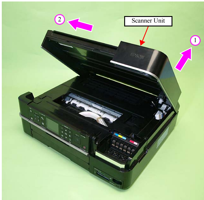
Figure 4-206. Removing the Scanner Unit (3)
