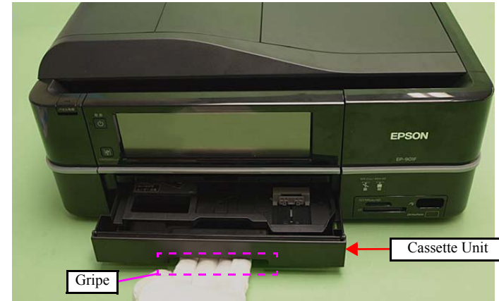
Figure 4-32. Removing the Cassette Unit
