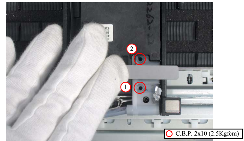
Figure 4-68. Assembling the Printhead (5)
