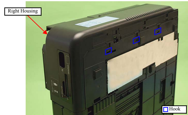
Figure 4-29. Removing the Right Housing/Card Cover (2)
