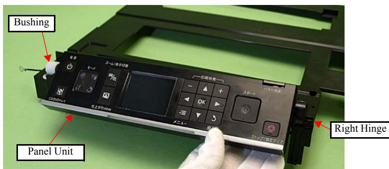
Figure 4-228. Removing the Panel Unit (3)
