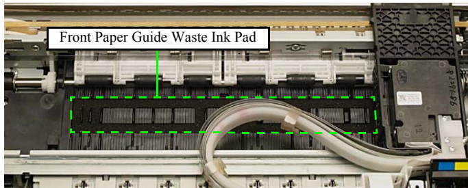
Figure 4-160. Removing the Front Paper Guide Waste Ink Pad
