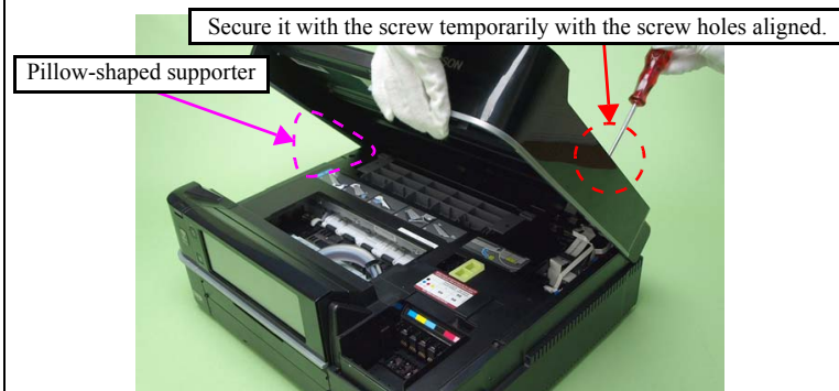
Figure 4-10. Installing the Scanner Unit (2)
