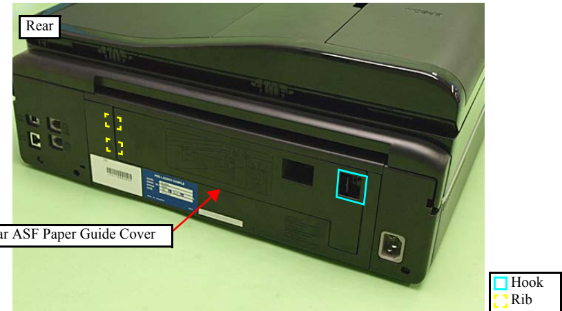
Figure 4-25. Removing the Rear ASF Paper Guide Cover
